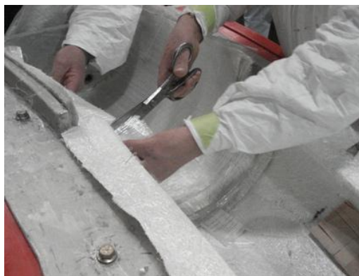
Fig. 37 Manual cutting of excess fabric during the manufacturing process
